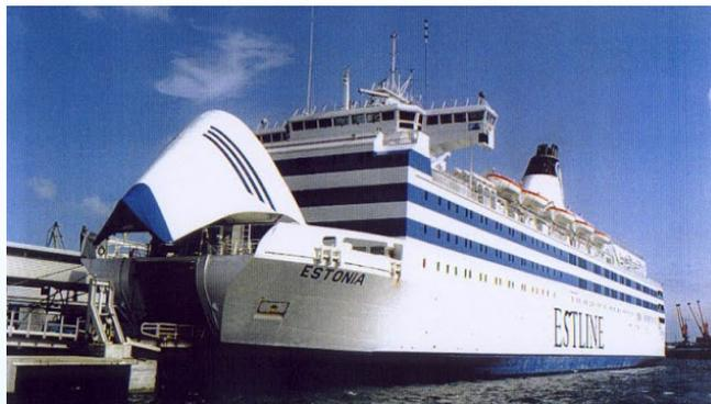
when it was put into service carrying passengers across the Baltic Sea between Tallinn, Estonia and Stockholm, Sweden. One unique feature of the ship would play a role in its demise. The ship had a bow door that swung upward to allow deployment of a vehicle ramp.
